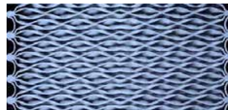
Cross section of plate pack
